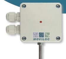
Controls the trailer temperature in real-time over the Internet, avoiding interruptions to the cold chain. Alarms can be displayed when values exceed preset limits.
